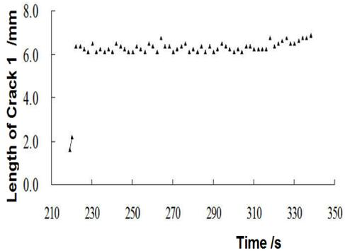
Figure 8. Variations in lengths of crack 1 with time at speeded failure stage.
