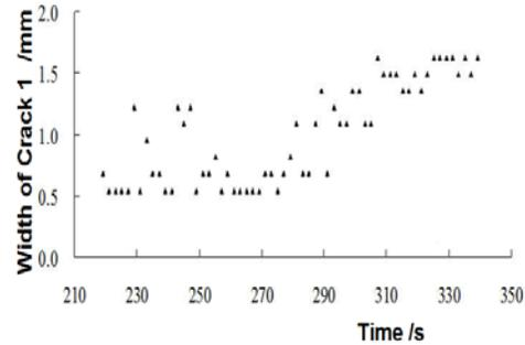
Figure 7. Variations in widths of crack 1 with time at speeded failure stage.
