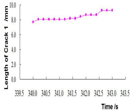
Figure 11. Variations in lengths with time of crack 1 at complete failure stage.
