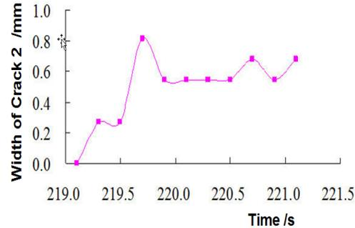
Figure 3. Variations in widths of crack 2 with time at stable stage.
