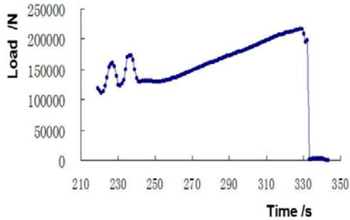
Figure 6. Variations in loads with time at speeded stage.
