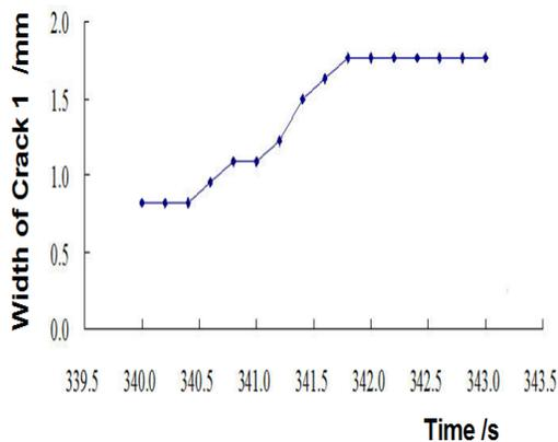
Figure 12. Variations in crack widths with time at 1.59 mm from the top tip of crack 1 at complete failure stage.
