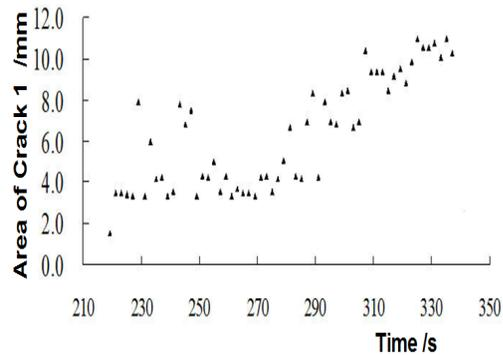
Figure 9. Variations in areas of crack 1 with time at speeded failure stage.
