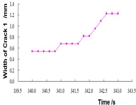
Figure 13. Variations in crack widths with time at 2.93 mm from the top tip of crack 1 at complete failure stage.
