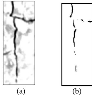
**Fig. 3** Newly-generated fissure distributions in granite image: (a) using fractional differential treatment; and (b) using threshold technique
