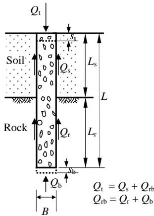
FIG. 1. Parameters considered for a test rock-socketed shaft.
