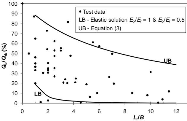
**FIG. 4. Variation of  $Q_b/Q_{rb}$  with  $L_r/B$  – test data and lower and upper bounding curves.**
