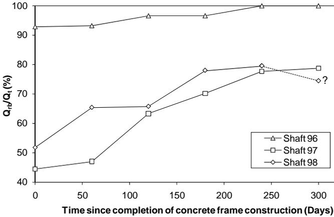
FIG. 7. Increase of rock-socket resistance with time (data from Tang 1995).
