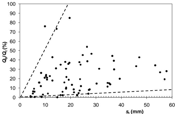
FIG. 6. Variation of  $Q_b/Q_t$  with shaft head displacement  $s_t$ .
