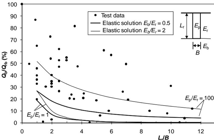
FIG. 3. Variation of  $Q_b/Q_{rb}$  with  $L_r/B$  – test data and elastic solutions of Rowe and Armitage (1987).
