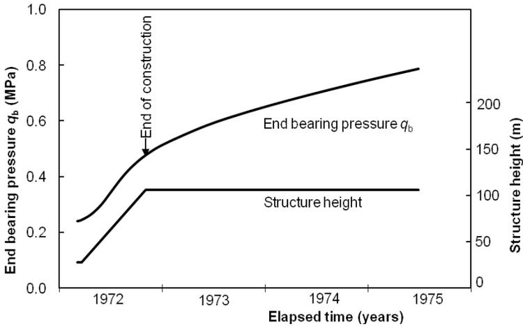
FIG. 8. End bearing resistance increase with time (data from Ladanyi 1977).
