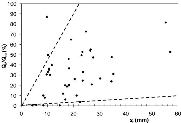
**FIG. 5. Variation of  $Q_b/Q_{rb}$  with shaft head displacement  $s_t$ .**
