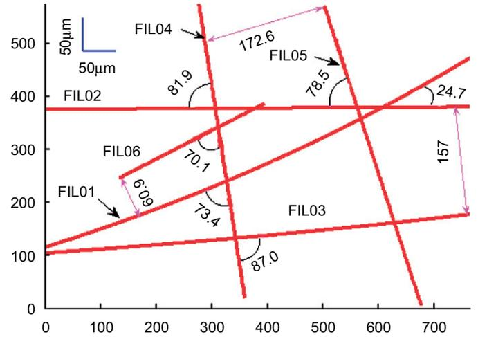
Fig. 8. Two types of FILs: parallel and intersecting.
