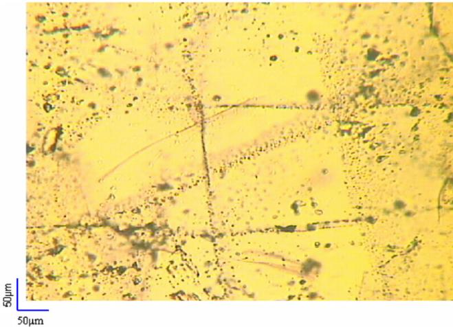
Fig. 1. An original image of fluid inclusions.
